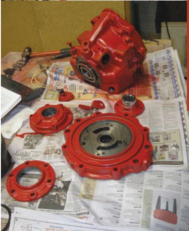
From the top: the fully deconstructed transmission, freshly repainted case parts and shiny new clutch disks. Opposite: the all-important owner's manual
