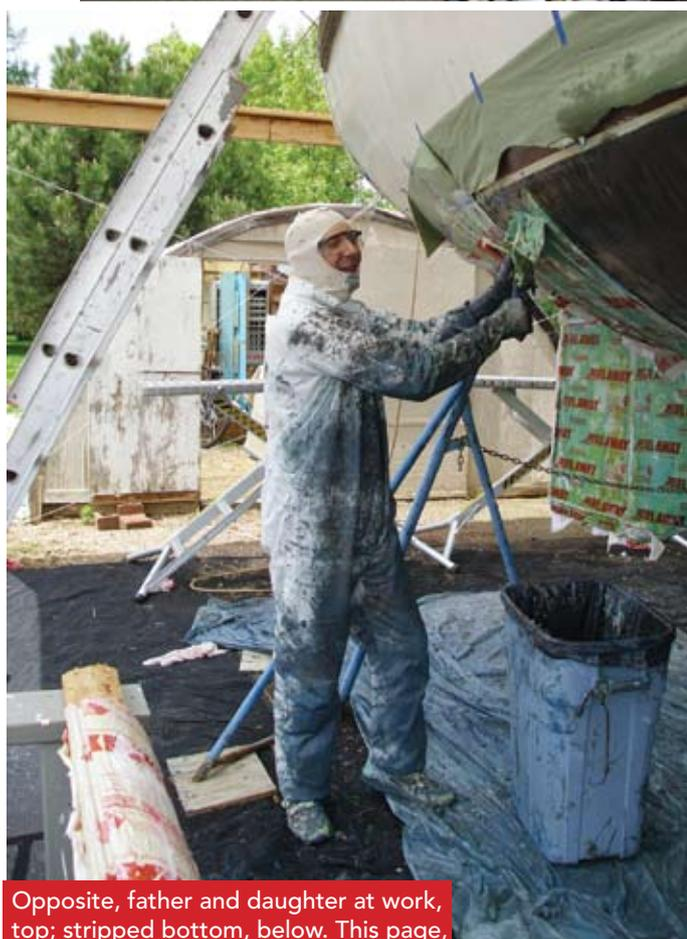
Opposite, father and daughter at work, top; stripped bottom, below. This page, from top: covering stripper with Peel Away sheeting; marine safety strip in place; removing the Peel Away
