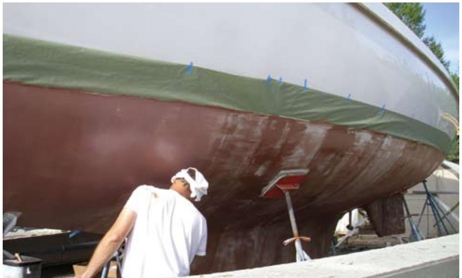
foam roller. As soon as the primer was not sticky (about three to four minutes) the silicone polymer-based topcoat was applied, but only with a brush. It is best to do the job in small sections so the primer does not dry for more than a few minutes before the topcoat is applied. The science here is that the topcoat melts into the primer, forming a well-adhered but very slick, very smooth, very shiny finish.
